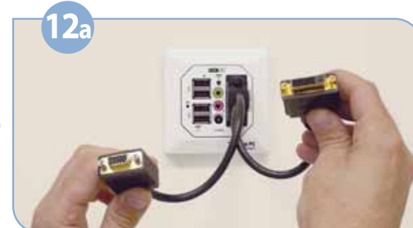
Some models offer dual-screen support. In order to get this functionality, connect Y-cable to the DVI monitor port. The Y-cable is to be purchased separately as accessory from Chip PC.
