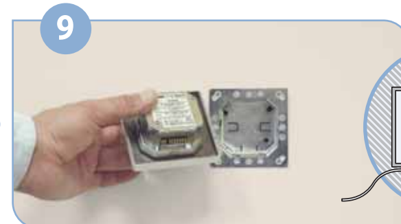
The Jack PC device should be inserted with contacts shown in picture facing downwards enabling direct contact with the Housing contacts.
