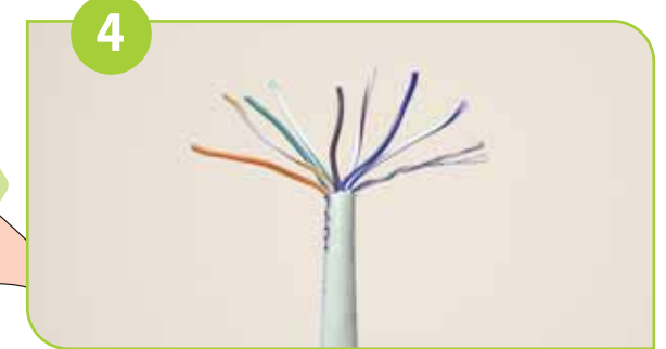
Pull out the LAN cable and remove 4cm/1.5 inch of its plastic insulation. Separate wire pairs by color.
