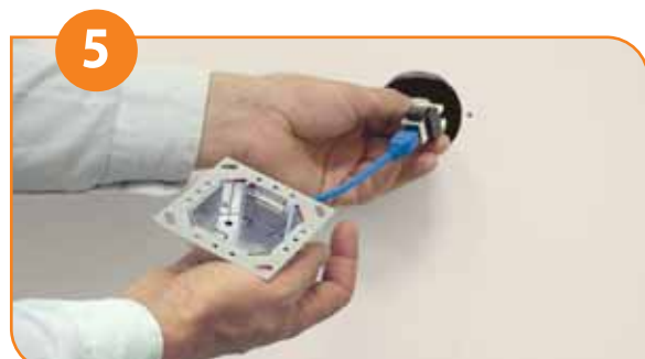
Insert the RJ-45 Termination Connector Block into the Housing bottom part until you hear a clicking sound indicating it has locked properly into place.
