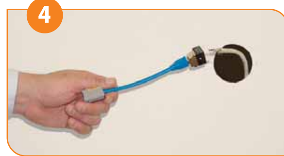
Connect the LAN jack and RJ-45 connector on the RJ-45 Termination Connector Block.
