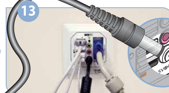
To power the device from an external power source, connect Chip PC-supplied power supply to the DC power jack. The power supply is to be purchased separately as accessory from Chip PC.
