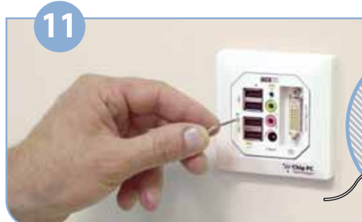
Note: in case you need to remove device after it was installed, unlock device by using the Extraction Tool turned clockwise.
