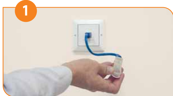
Use Power-over-Ethernet tester to check existence of PoE in the Jack designated for installation. Note: In case there is no PoE available, Jack PC can be powered by External power supply (see step 13).
