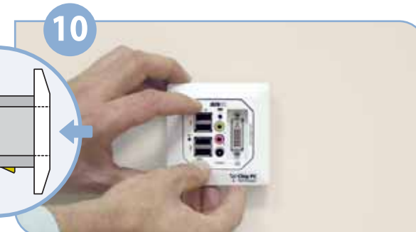
Insert the Jack PC device into the Housing until you hear a clicking sound indicating the device has locked properly into place. Verify locking by gently pulling device outwards.
