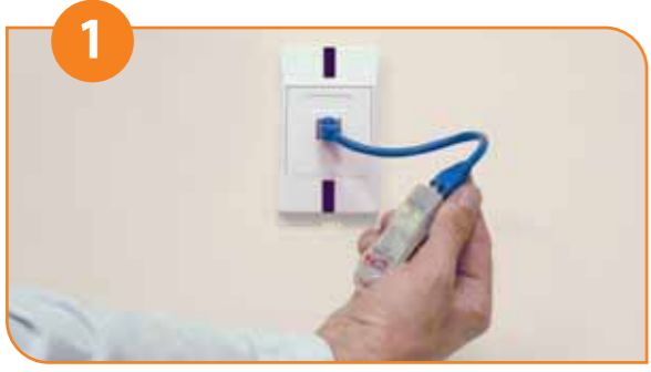
Use Power-over-Ethernet tester to check existence of PoE in the Jack designated for installation. Note: In case there is no PoE available, Jack PC can be powered by External power supply (see step 13).
