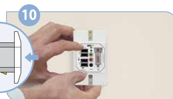
Insert the Jack PC device into the Housing until you hear a clicking sound indicating the device has locked properly into place. Insert additional 2 screws to the frame and tighten.
