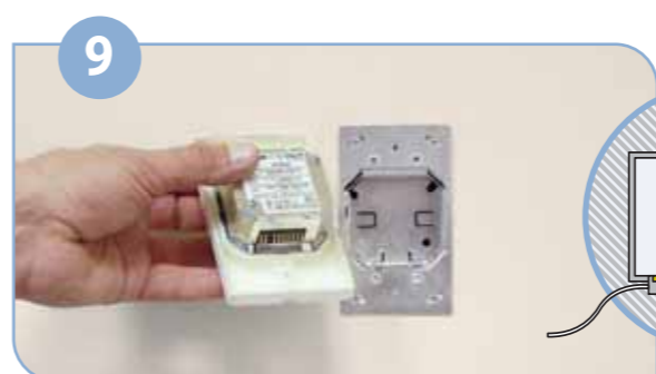
The Jack PC device should be inserted with contacts shown in picture facing downwards enabling direct contact with the Housing contacts.
