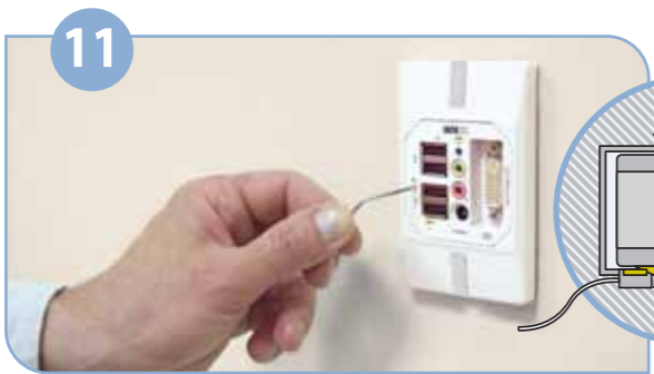
Note: In case you need to remove device after it was installed, remove the 2 screws from frame and unlock device using the Extraction Tool turned clockwise.
