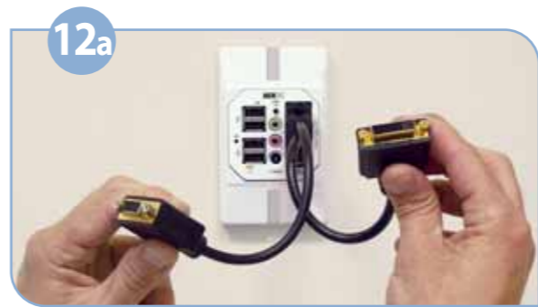
Some models offer dual-screen support. In order to get this functionality, connect Y-cable to the DVI monitor port. The Y-cable is to be purchased separately as accessory from Chip PC.
