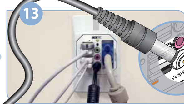
To power the device from an external power source, connect Chip PC-supplied power supply to the DC power jack. The power supply is to be purchased separately as accessory from Chip PC.
