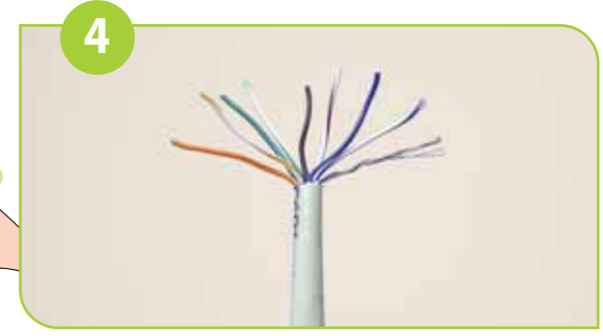
Pull out the LAN cable and remove 4cm/1.5 inch of its plastic insulation. Separate wire pairs by color.
