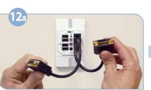
Some models offer dual-screen support. In order to get this functionality, connect Y-cable to the DVI monitor port. The Y-cable is to be purchased separately as accessory from Chip PC.
