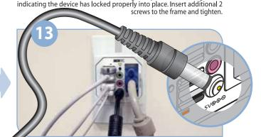
To power the device from an external power source, connect Chip PC-supplied power supply to the DC power jack. The power supply is to be purchased separately as accessory from Chip PC.
