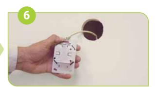
Close the IDC Krone Termination Connector Block and insert it into the Housing bottom part until you hear a clicking sound indicating it has locked
