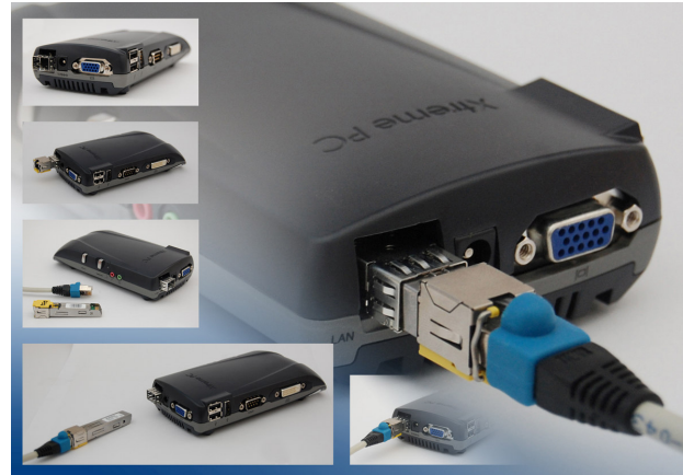
Xtreme PC LXN 2321F with CAT 5 Network Interface
