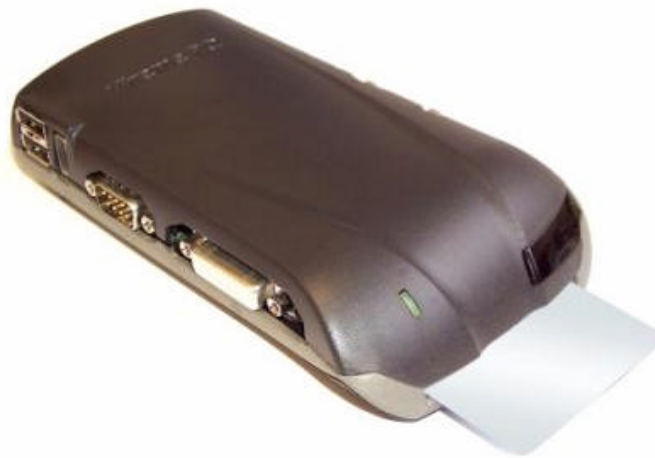
Figure 9: Xtreme PC with Built-in PC/SC Smart Card Reader
